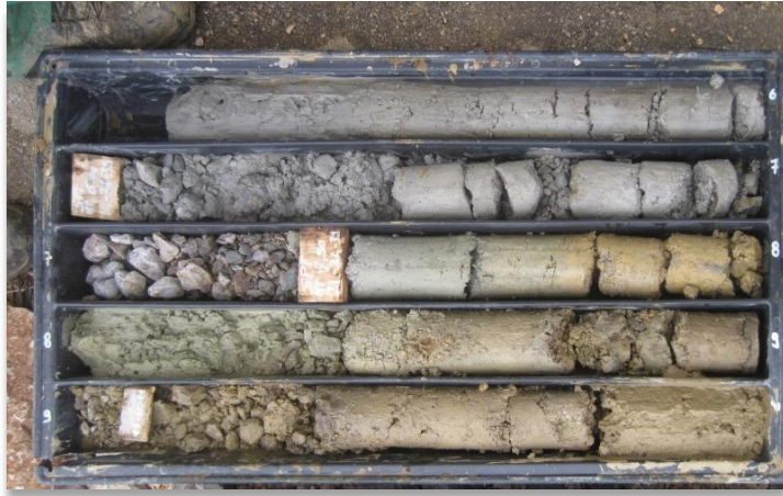
Borehole core samples © BBB, 2014
